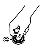
Line up openings in the reflector bowl with the surface unit receptacle and the element holddown clip.
